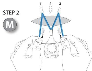
With the next movement form the letter **M** by guiding the tension line around tabs #4 and #6.
