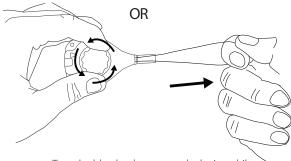
Turn the blue knob counter-clockwise while pressing down on the knob.
