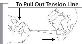
Press down on the center of the tension controller knob while pulling the line out with the other hand.
